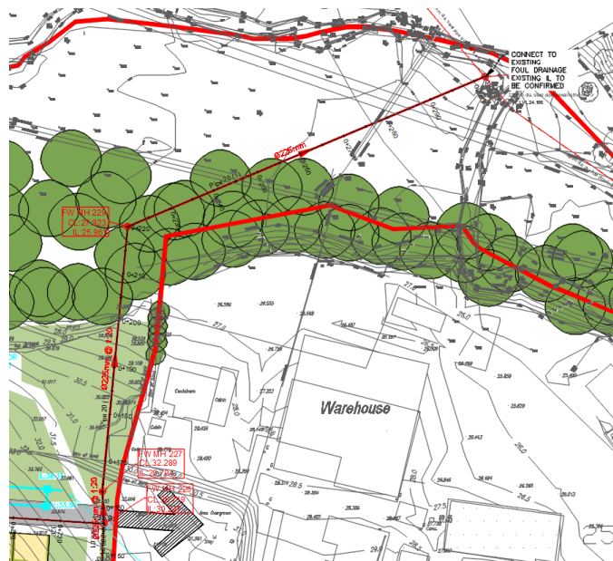
Figure 2: Proposed Gravity Foul Sewer Towards Three Trout Stream
